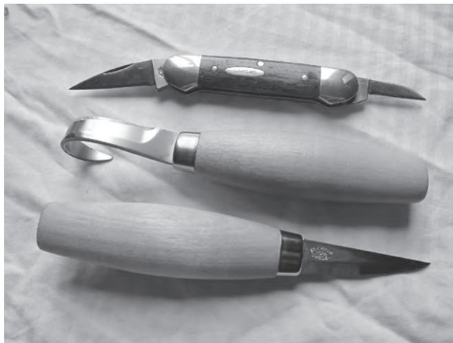
out the bowl. I recently began using a Flexcut Pocket Jack for Carvin' when carving away from home. (At home I use a Mora 3" fixed-blade wood carving blade and a Mora hook-knife for the
