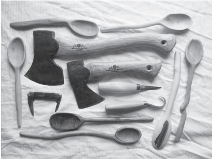
The hatchet is used to split the limb and provide spoon-blank shaping. I let the grain twists and turns of the shrub's growth pattern determine the design of the spoon. I use a Gransfors Bruks carving axe for the quick shaping and the "Kubben" hand hatchet for tight, exacting work of a spoon. The "Kubben" comes with a forged
